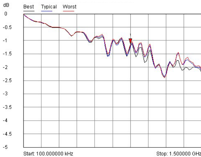
60-731 Typical Insertion Loss
